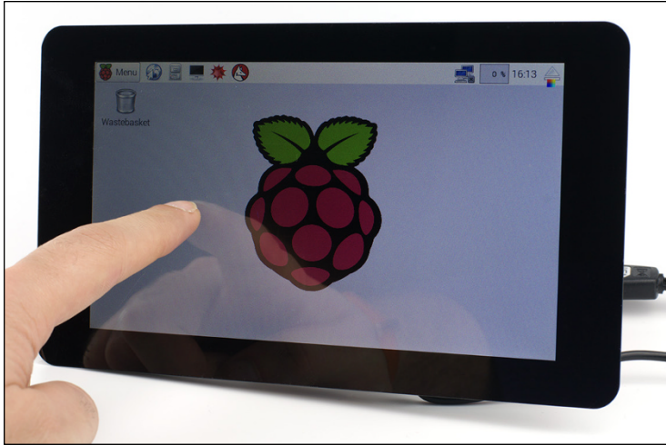
FIGURE 16-4: Using the Raspberry Pi 7" touchscreen display
